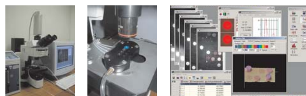
Figure 3: Setup of microscope CCD detection system, thermostated hybridization chamber and PamChip Analyzer Data Analysis package
